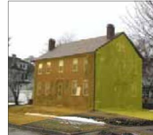
A corner lot typically has two façade zones, one for each public street.
